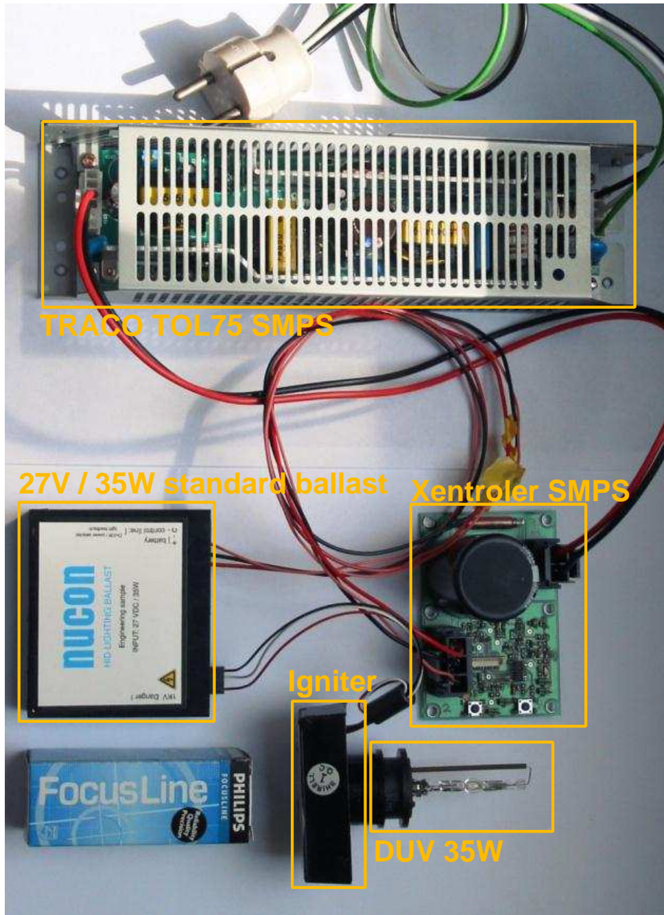
picture 4: Application example: Using special programmed Xentroler SMPS in combination with Traco TOL75 switching mode power supply to drive UV bulb of Philips MPXL Focusline with standard 27V/35W ballast and igniter system. The standard quick start is cut back by the Xentroler to avoid damage of electrodes during warm up phase. Application of Xentroler SMPS enables application of low cost standard components to obtain reasonable overall system cost for the special DUV 35W bulb.
